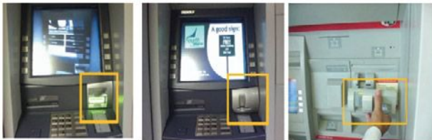
(A) Normal card entry interface (B) Skimming device at card entry interface (C) Skimming device 'Piggy Backed' onto card reader
